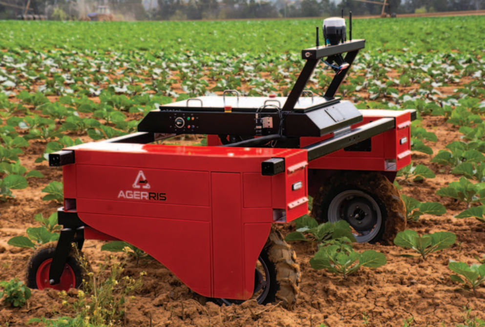
Robots such as Agerris' Digital Farmhand carry out targeted mechanical and chemical weeding with precise control capability. Agerris
